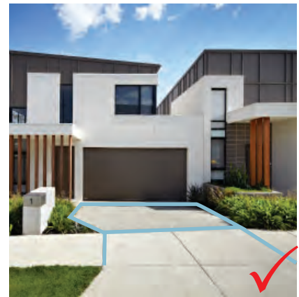
Figure 34 – Textured concrete surface with tapering to match crossover
