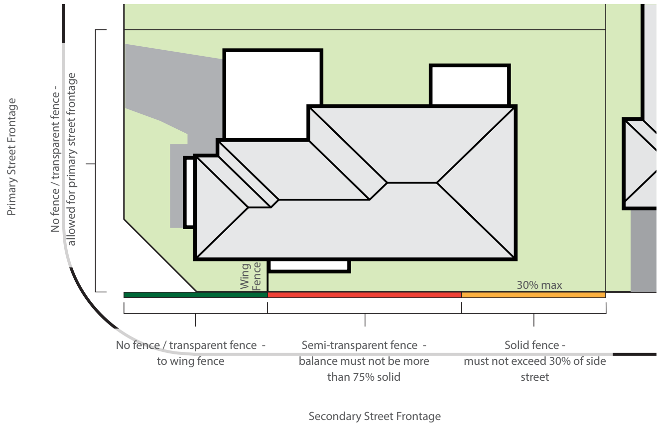
Figure 40 – Side street fencing on corner allotments
